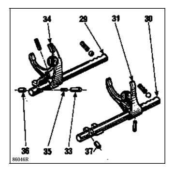
Retrieve the interlock plunger (35) located in the 1st/2nd shaft as well.
