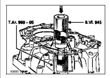
The guide tube lubrication hole is lower down than the housing hole.
