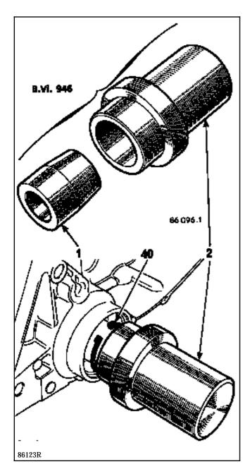
The seal is refitted using tool **B. Vi. 945** made up of:
