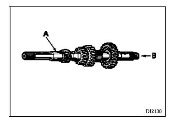
On shafts which have a jet (B), this cannot be removed. Clean the 5th gear lubrication hole.
