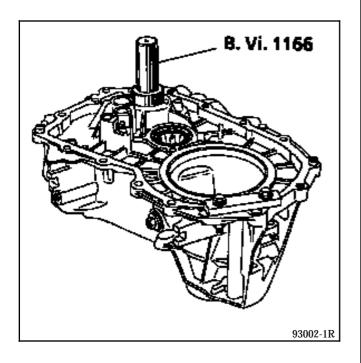
The mechanism housing twin bearing outer races are fitted using tool **B. Vi. 1164** or equivalent.
