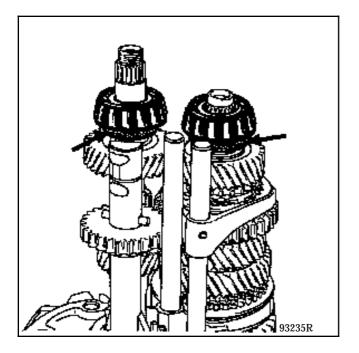
Fit the 1/2 and 3/4 locking balls and springs in the mechanism housing then fit the 13 mm diameter dummy shafts (A).
