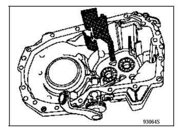
Push as far as possible and check the clipping of the retainer (A).
