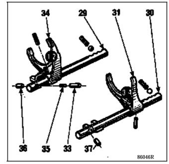
Fit the assembled 1/2 shaft and fork to the 1/2 sliding gear of the assembled output shaft, fitted with the locking plunger **(35)**.
