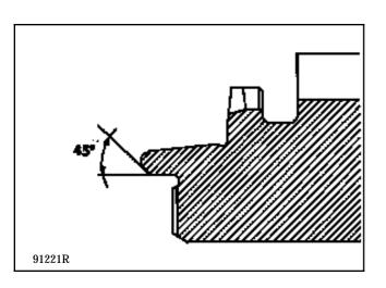
The  $45^{\circ}$  input chamfer (E) for the groove and tongue joint under the synchronisation cone will only allow the fitting of "Z"-shaped springs.
