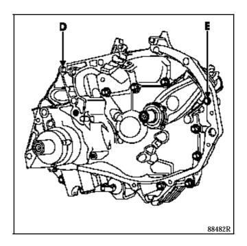
If necessary, remove the centring pins placed at (D) and (E).
