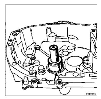
For guides without flanges (JB0 - 1 - 2 - 3), push down the part until it is flush with the gauge housing (marked by the ring position graduation on the tube).
