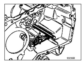
Apply **Loctite 518** to the mating surface between the clutch housing and the mechanism housing.
