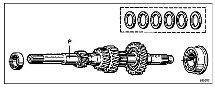
As the lip seal is in direct contact with the input shaft, check the condition of mating surface P. If there are any scratches or faults in appearance, change the input shaft.
