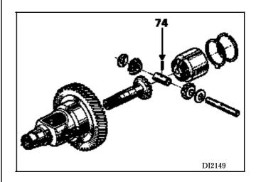
It is essential to fit a new pin (74) (using tool **B. Vi. 31-01**).
