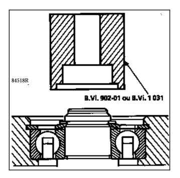
Fit the input shaft washer and fit the circlip by reaction, immobilising the shaft at the clutch splines end using bolt (T) of plate **B. Vi. 950-02**; ensure that the circlips are correctly fitted in the groove.
