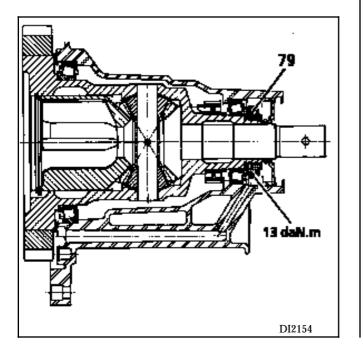
As on removal, immobilise the housing - crown wheel assembly using tool **B. Vi. 1 057** secured to the housing.
