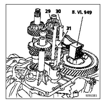
Place the 1/2 shaft (29) and the reverse gear (32) in neutral).
