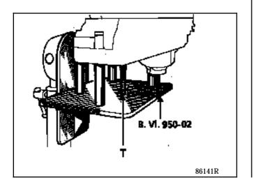
**4-speed gearbox:** change the threaded thrust pad.
