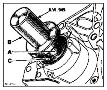
**NOTE:** the lip seal can be changed on the vehicle with the gearbox in place.
