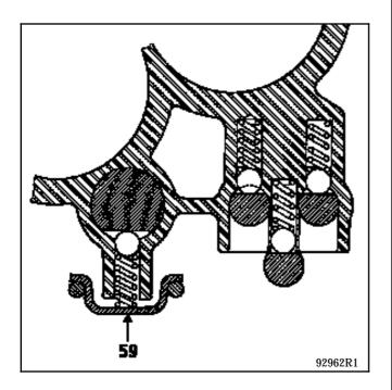
It is advisable to fit two magnets or to close the openings (C) in order to retrieve the locking springs and balls of the 1/2 and 3/4 shafts.
