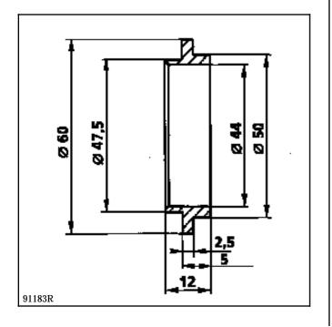
Spacer assembled on a differential housing fitted on TAPERED BEARINGS .
