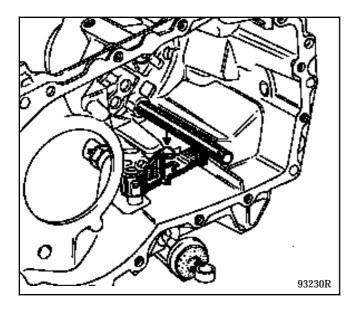
Detach and raise the mechanism housing fitted with the 5th gear shaft.
