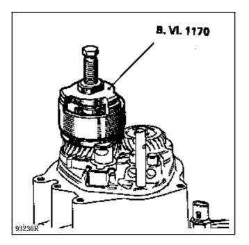
Remove the 5<sup>th</sup> gear fork and sliding gear.
