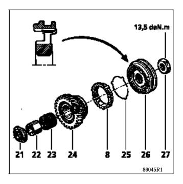
In order to allow the input and output shaft nut and bolt to be tightened to the specified torque, the two 5<sup>th</sup> gears must be fitted and two gears must have been engaged.
