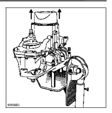
Remove the rear housing. This must be removed in the horizontal centreline of the gearbox as it has a lubrication nozzle located in the input shaft bore.
