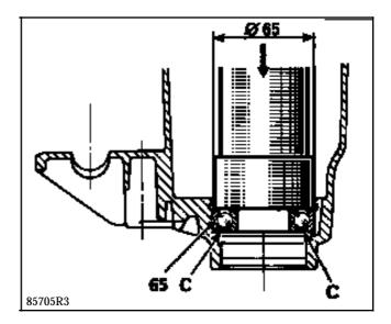
Change the bearing retaining circlips.
