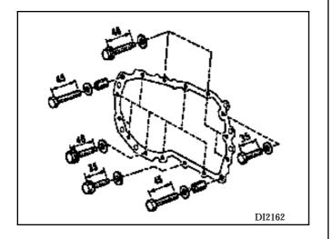
Tighten the peripheral bolts to the specified torque after turning the input shaft to ensure correct final coupling of the cones on the tapered rollers.
