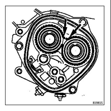
Fit the bearings to tools **B. Vi. 947** (JB0 - JB1 - JB2 - JB3) or **B. Vi. 1 030** (JB4 and JB5), groove at the opposite end to the input cone.
