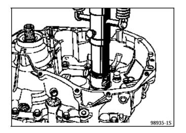
For guides with flanges (JB4 and 5), fit as far as possible using a press.
