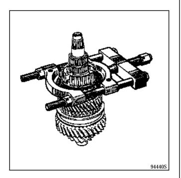
Using a press, remove theinner hubs, 1<sup>st</sup> and 2<sup>nd</sup> gears, hub, sliding gear assembly, taking the load under the 1<sup>st</sup> gear.
