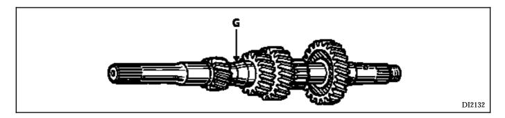
On **JB2** gearboxes, this modification is accompanied by the fitting of sealed bearings (Ø 62 mm).
