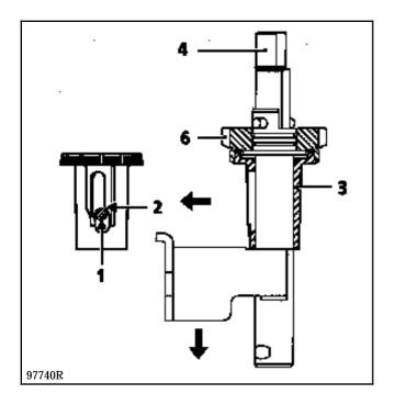
This device, which complements the reverse gear brake, allows the gear to be engaged with no impact of the teeth.
