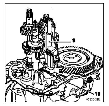
Lifting the reverse gear guide (9), the end is disengaged from its seat (10).
