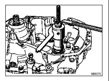
Fit the sheath and the split ring and then gently extract the guide tube acting on the upper nut (B).
