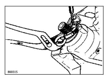
Immobilise the differential housing - crown wheel assembly using tool **B. Vi. 1 057** secured to the housing.
