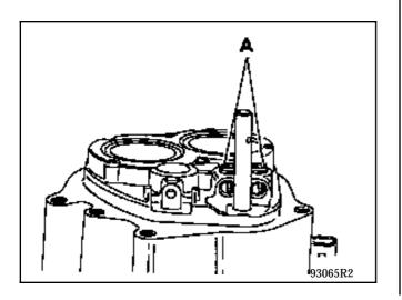
Fit the 5<sup>th</sup> gear locking ball and spring in the mechanism housing then place the 5<sup>th</sup> gear fork shaft (B) in neutral.
