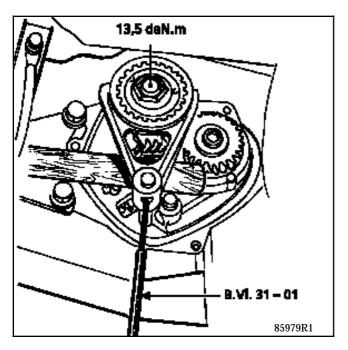
Observe the direction of fitting, the split must be directed towards the rear housing.
