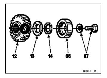
Fit the washer (13) and the circlip (14) : tool **B. Vi. 948** or equivalent.
