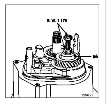
Remove tool **B. Vi. 1175** and fit bolt (65) coated with 3 drops of Loctite FRENBLOC.
