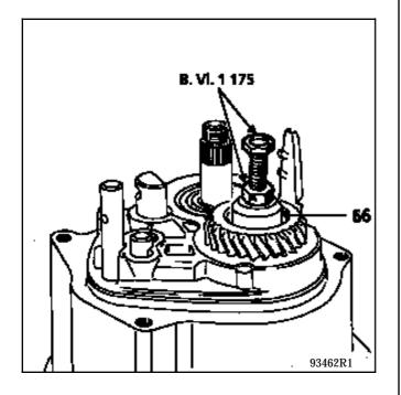
Remove tool B. Vi. 1 175 and the washer (66).
