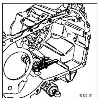
Observe the direction of the pins, their slits must be perpendicular to and opposite the shaft.
