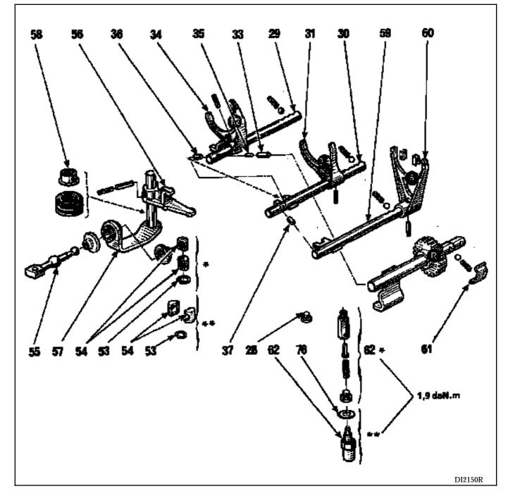
The shafts must not be deformed and the locking balls seat must not be worn. The locking balls must also slide freely in their bearings without excessive clearance.
