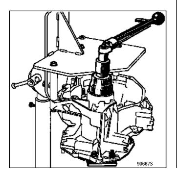
Remove tool **B. Vi. 1057** and turn the differential to position the bearings.
