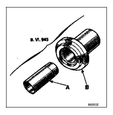
Fit the protector (A) coated with oil to the sun wheel and position the seal (C) coated with oil using tool (B).
