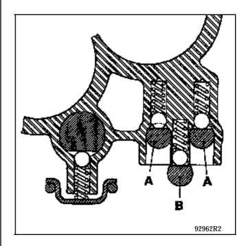
Check the position of the  $5^{\text{th}}$  gear lubrication channel and the breather.
