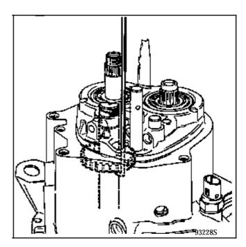
Fit the locking ball, its spring and the retaining Uclip **(59)**.
