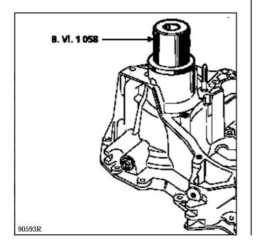
Fit the O-ring on the sun wheel and coat the splines with MOLYKOTE "BR2" grease.
