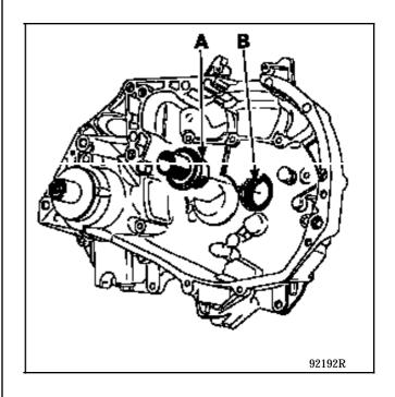
Insert the guide tube using a press until it is in contact with the external surface of the housing.
