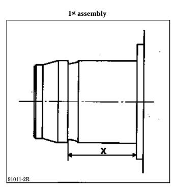
Assembly with spring washer "R"  $\varnothing$  35.6 mm thickness 2.6 mm.
