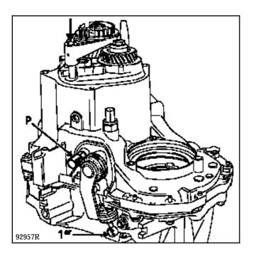
Remove the 5<sup>th</sup> gear detent (P).
