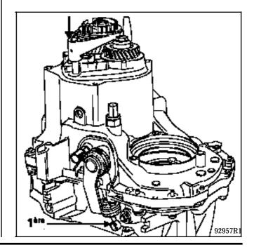
Apply 3 drops of **Loctite FRENBLOC** to input shaft nut (27) and the output shaft bolt.
