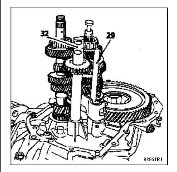
Simultaneously pull the two shafts (input - output) and the assembled 1/2 fork shaft, (29 and 34).
