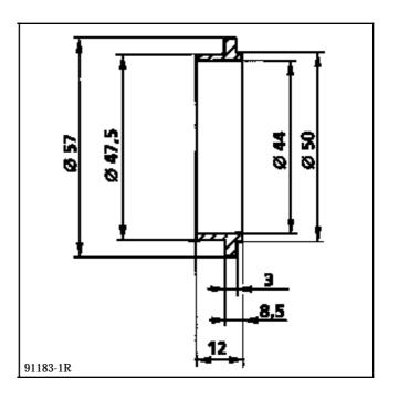
It is essential that the spacer which corresponds to the type of differential housing is fitted .
