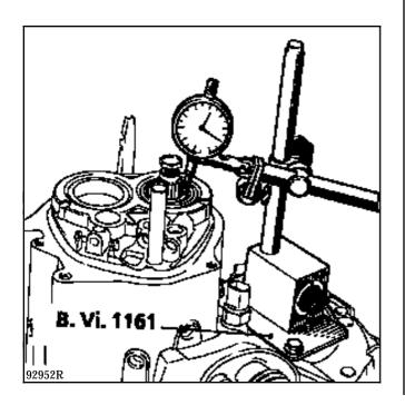
Fit the dial gauge with its magnetic base.
