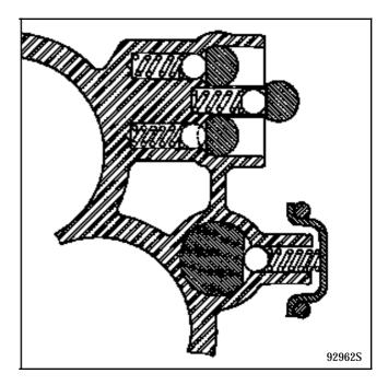
It is advisable to fit two magnets or to close the openings (C) in order to retrieve the 1/2 and 3/4 shaft locking balls and springs.
