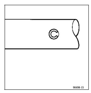
2) The pin must always be changed whenever it is removed.
